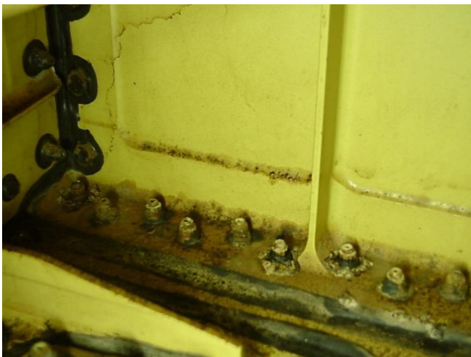
Figure 2 - Microbial growth on a fuel tank surface – note the contamination is seen on ledges on the tank walls not just on the tank bottom
