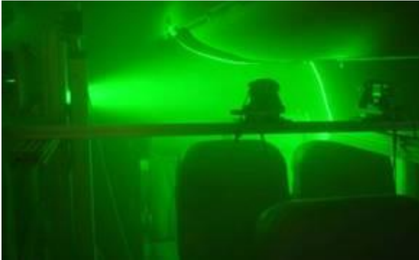
Measuring cabin air flow
